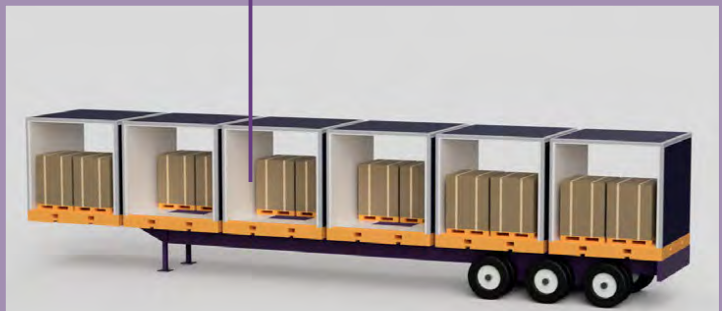
Active Delivery Mode - with Doors Open on either side for easier unloading from both sides.
